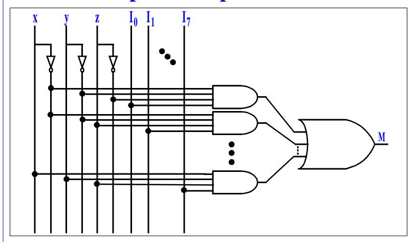
•M =  $x'y'z'I_0 + x'y'zI_1 + x'yz'I_2 + x'yzI_3$ +  $xy'z'I_4 + xy'zI_5 + xyz'I_6 + xyzI_7$
